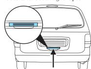
3. Pull up on the liftgate handle to engage the power assist feature. Release the handle as soon as the PLG begins to power open.
